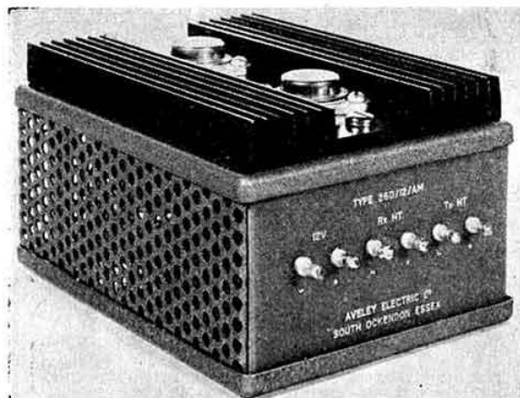
The Avel 130 watt d.c.-to-d.c. converter manufactured by Aveley Electric Ltd. The converter, which operates from a nominal 12 volt d.c. supply, provides outputs of 425 volts at up to 300 mA and 265 volts at 100 mA. It is thus suitable for providing power to a complete mobile station such as a K.V. Valiant transmitter and companion receiver.
