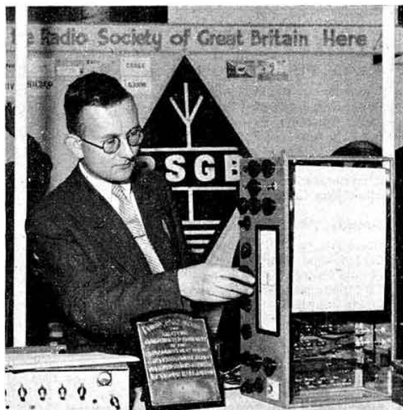
Mr. A. L. Mynett, G3HBW, received the Silver Plaque for the transistor communications receiver for the 430 and 1296 Mc/s bands shown in this picture. (Photo by Tella Photography Ltd.)
