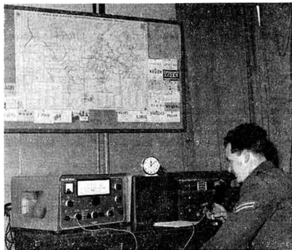
Cpl. George Stanton operating DL2VR, the club station of the 1st Signal Regiment in Germany. The transmitter is a K.W. Viceroy and the receivers include an AR88 and Eddystone 770. A Drake 2B is to be added shortly. Aerials include a Mosley three element beam for 15m, a cubical quad for 20m and dipoles for 40 and 80m.
